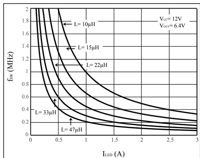
**Figure 34** Inductance Selection Based On 30% Current Ripple
