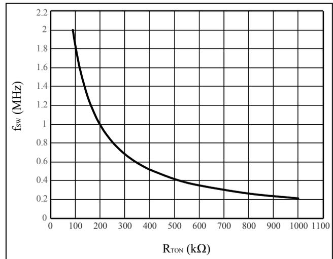
Figure 30 Operating Frequency vs. R<sub>TON</sub> Resistance
