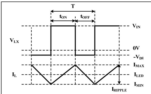
Figure 31 Operating Waveform
