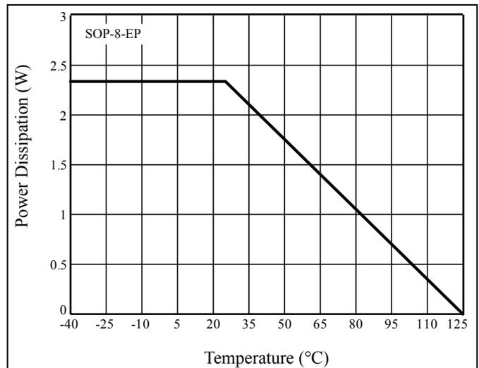
Figure 35 Dissipation Curve
