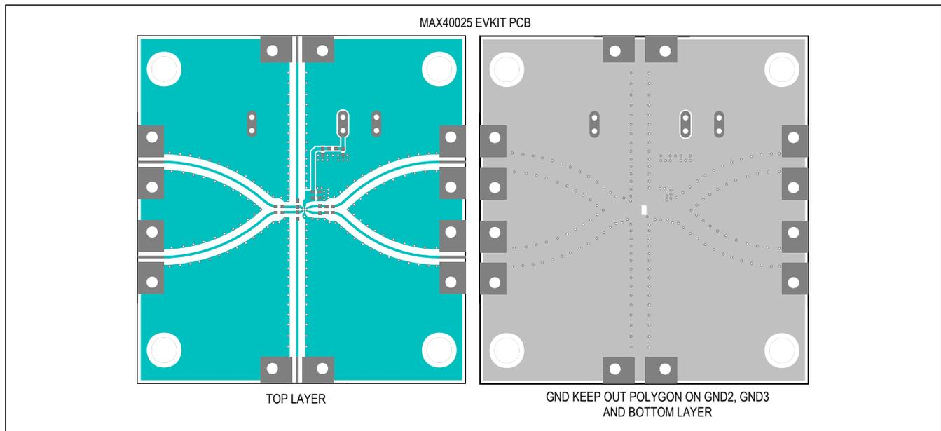
Figure 7. Layout Guidelines—Ground Keep-Out to Avoid Stubs.
