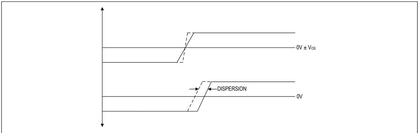
Figure 4. Slew Rate Dispersion
