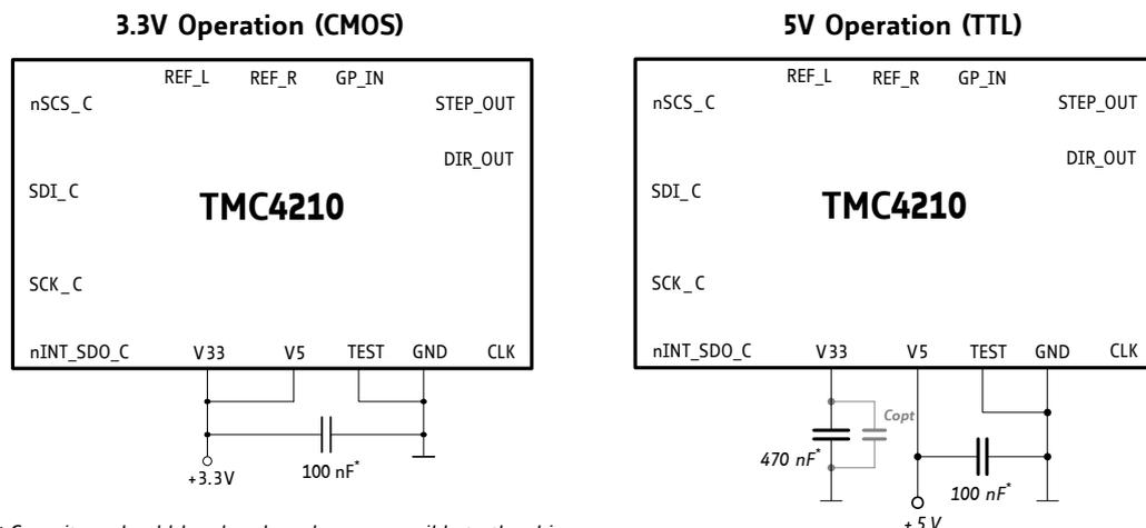
\* Capacitors should be placed as close as possible to the chip.
