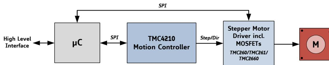
Figure 1.2 Application example using Step/Dir driver interface
