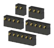
KYOCERA AVX has added a 90-degree version to its battery connector range. It is offered on a 3 mm pitch, in 2 to 6 contact positions, and is rated at 3 amps, as are all of the battery range. The small, compact design of the connector minimizes its profile while maintaining stability with a contact point 4.61 mm above the PCB.
