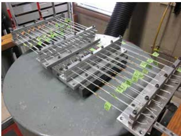
Figure 2 – Military Vibration Test - SOLISTRAND Splices
