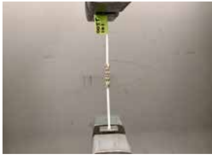
Figure 4 - Crimp Tensile Strength Test - Diamond Grip Butt Splice
